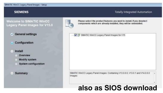
**Note:** The Panels can be configured, created and simulated in the TIA Portal even if the Image/Runtime is not installed. These are required however for downloading the device or the ProSave functions
