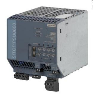
SITOP PSU8600/3AC/24VDC/40A/4X10A PN SITOP PSU8600 3AC 40A/4x10A PN Stabilized power supply Input: 400-500 V 3 AC output: 24 V DC/40 A/4x 10 A with PN/IE connection Integrated web server OPC UA server integrated
