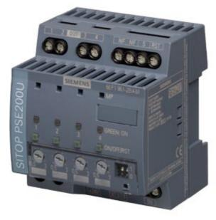
SITOP PSE200U SELECTIVITY MODULE 3A SITOP PSE200U 3 A NEC CLASS 2 Selectivity module 4-channel input: DC 24 V/12 A output: 24 V/4x 3A NEC class 2 Level adjustable 0.5-3 A mit status message for each output
