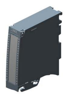
SIMATIC S7-1500, digital output module DQ16x24 V DC/0.5 A HF; 16 channels in groups of 8; 4 A per group; Single-channel diagnostics; Substitute value: Front connector (screw terminals or push-in) to be ordered separately
