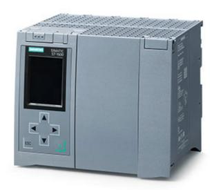
SIMATIC S7-1500F, CPU bundle Consisting of: CPU 1518F-4 PN/DP MFP (6ES7518-4FX00-1AB0), including C/C++ Runtime and OPC UA Runtime license, work memory 6 MB for program and 20 MB for data, 1st interface: PROFINET IRT with 2-port switch, 2nd interface: PROFINET RT, 3rd interface: PROFINET basic services, 4th interface: PROFIBUS, 1 ns bit performance, SIMATIC memory card (min. 2 GB) required
