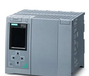
SIMATIC S7-1500F, CPU 1518F-4 PN/DP, Central processing unit with work memory 6 MB for program and 20 MB for data, 1st interface: PROFINET IRT with 2-port switch, 2nd interface: PROFINET RT, 3rd interface: PROFINET basic services, 4th interface: PROFIBUS, 1 ns bit-performance, SIMATIC Memory Card required
