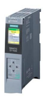
SIMATIC S7-1500F, CPU 1511F-1 PN, CENTRAL PROCESSING UNIT WITH WITH WORKING MEMORY 225 KB FOR PROGRAM AND 1 MB FOR DATA, 1. INTERFACE: PROFINET IRT WITH 2 PORT SWITCH, 60 NS BIT-PERFORMANCE, SIMATIC MEMORY CARD NECESSARY
