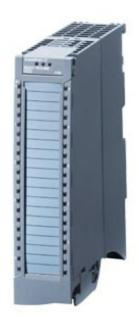
SIPLUS S7-1500 AI 8xU/I HS TX RAIL -40 ... +70°C TX with 85°C for 10 min with conformal coating based on 6ES7531-7NF10-0AB0 . 16 Bits of Resolution, Accuracy 0.3 "Percent; 8 Channels in Groups" "of 8; Common Mode Voltage" "Appr.10V; Diagnosis," "Processalarms; 8 Channels in" 0.0625 ms incl. Infeed element, Shield Clamp and Shield Terminal
