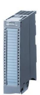
SIPLUS S7-1500 DI 16x110VDC HF TX RAIL -40 ... +70°C TX with 85°C for 10 min with conformal coating based on 6ES7521-7EH00-0AB0 . DI 16x24 ... 125V UC HF, 16 channels in groups of 1 Input delay 0,05 ... 20ms Input type 3 (IEC "61131); diagnostics, Hardware" interrupts
