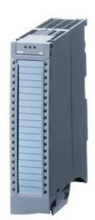
SIPLUS S7-1500 AQ 8xU/I HS -40...+70 °C Start up -25 °C with conformal coating based on 6ES7532-5HF00-0AB0 . Analog output module AQ8xU/I HS, 16 bit resolution, Accuracy 0.4%, 8 channels in groups of 8, "diagnostics; substitute value" 8 channels in 0.125 ms incl. infeed element, Shield bracket and shield terminal
