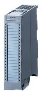
SIPLUS S7-1500 AI 8xU/I HS -40 °C ... +70°C with conformal coating based on 6ES7531-7NF10-0AB0 . Analog input module AI 8xU/I HS, 16 bit resolution, Accuracy 0.4% 8 channels in groups of 8, "Common mode voltage 10 V;" "diagnostics; hardware" "interrupts"" 8 channels in 0.125" ms incl. infeed element, Shield bracket and shield terminal
