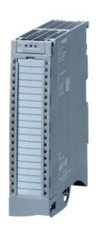
SIPLUS S7-1500 AI 8XU/I HF -40 ... +70°C with conformal coating based on 6ES7531-7NF00-0AB0 . 16 bit resolution, Accuracy 0.1%, 8 channels in groups of 1, Common mode voltage: 30V AC/60V DC, "diagnostics; hardware" "interrupts; incl. infeed" element, Shield bracket and shield terminal
