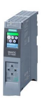
SIPLUS S7-1500 CPU 1513F-1 PN -25+60°C with conformal coating based on 6ES7513-1FL02-0AB0 . Central processing unit with work memory 450 KB for program and 1.5 MB for data, 1st interface: PROFINET IRT with 2-port switch, 40 ns bit performance, SIMATIC Memory Card required
