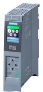
SIPLUS S7-1500 CPU 1513-1 PN -40°C+60°C with conformal coating based on 6ES7513-1AL02-0AB0 . Central processing unit with Work memory 300 KB for program and 1.5 MB for data, 1st interface: PROFINET IRT with 2-port switch, 40 ns bit performance, SIMATIC Memory Card required
