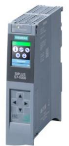
SIPLUS S7-1500 CPU 1511-1 PN -40°C+60°C with conformal coating based on 6ES7511-1AK02-0AB0 . Central processing unit with Work memory 150 KB for program and 1 MB for data, 1st interface: PROFINET IRT with 2-port switch, 60 ns bit performance, SIMATIC Memory Card required
