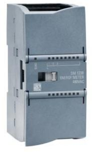
SIMATIC S7-1200, Analog input, SM 1238 Energy Meter 480 V AC, power measurement module for data acquisition in 1- and 3-phase supply systems (TN, TT) up to 480 V AC; Current range: 1 A, 5A; acquisition of voltage, current, phase angles, power, energy values, frequencies; Channel diagnostics
