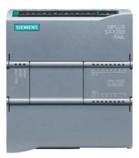
SIPLUS S7-1200 CPU 1212C DC/DC/DC T1 RAIL -25 ... +55°C T1 with 70°C for 10 min with conformal coating based on 6ES7212-1AE40-0XB0 . compact CPU, DC/DC/DC, Onboard I/O: 8 DI 24 V DC 6 DO 24 V DC 2 AI 0-10 V DC, Power supply: 20.4-28.8V DC Program/data memory 50 KB
