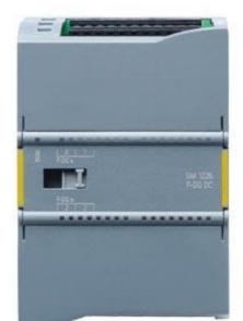
SIPLUS S7-1200 SM 1226 F-DQ 2x relay -25...+55°C with conformal coating based on 6ES7226-6RA32-0XB0 . F-DQ 2x RLY 5A, PROFIsafe, 70 mm overall width, up to PL E (ISO 13849-1)/ SIL3 (IEC 61508)
