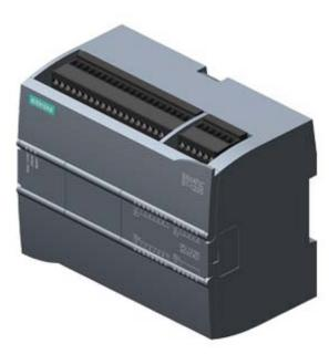
SIPLUS S7-1200 CPU 1215C AC/DC/relay -40...+70°C with conformal coating based on 6ES7215-1BG40-0XB0 . compact CPU, AC/DC/relay, 2 PROFINET Port,onboard I/O: 14 DI 24 VDC 10 DO relay 2 A 2 AI 0-10 VDC 2 AO 0-20 mA DC Power supply: 85-264V AC @ 47-63 Hz, Program/data memory 125 KB
