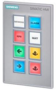
SIPLUS HMI KP8F PN -20...+55°C with Conformal Coating based on 6AV3688-3AF37-0AX0 . Key Panel, 8 short-stroke switches with multi-colored LEDs, PROFINET interfaces with PROFIsafe; 8 DI/DO and 2 safety DI pins, 24 V DC can be looped through parameterizable as of STEP 7 V5.5
