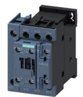
Contactor, AC-1, 50 A/400 V/40  $^\circ\text{C},$  S0, 4-pole, 230 V AC/50 Hz, 1 NO+1 NC, screw terminal
