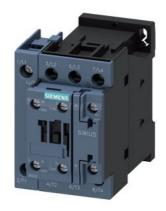
Contactor, AC-1, 40 A/400 V/40  $^{\circ}\text{C}$  , S0, 4-pole, 230 V AC/50 Hz, 1 NO+1 NC, screw terminal
