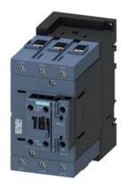
power contactor, AC-3 110 A, 55 kW / 400 V, 1 NO + 1 NC, 24 V AC, 50 Hz 3-pole, 3NO, Size S3 screw terminal
