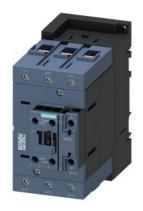
power contactor, AC-3 95 A, 45 kW / 400 V 1 NO + 1 NC, 110 V AC, 50 Hz 3-pole, 3 NO, Size S3 screw terminal
