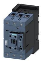
power contactor, AC-3 80 A, 37 kW / 400 V 1 NO + 1 NC, 20-33 V AC/DC 3-pole, 3 NO, Size S3 screw terminal integrated varistor
