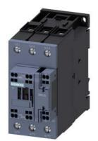
Contactor, AC-3, 37 kW / 400 V, 1 NO + 1 NC, 110 V AC, 50 Hz, 3-pole, Size S2, Spring-type terminal
