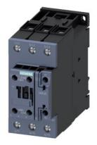
Power contactor, AC-3 80 A, 37 kW / 400 V 1 NO + 1 NC, 20-33 V AC/DC with varistor 3-pole, size S2 screw terminals
