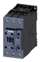
Power contactor, AC-3 80 A, 37 kW / 400 V 1 NO + 1 NC, 230 V AC, 50 Hz 3-pole, size S2 screw terminals
