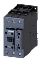
Power contactor, AC-3 80 A, 37 kW / 400 V 1 NO + 1 NC, 24 V AC, 50 Hz 3-pole, size S2 screw terminals
