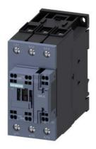
power contactor, AC-3 50 A, 22 kW / 400 V 1 NO + 1 NC, 230 V AC, 50 Hz 3-pole, Size S2, Spring-type terminal
