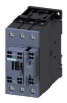
power contactor, AC-3 50 A, 22 kW / 400 V 1 NO + 1 NC, 24 V AC, 50 Hz 3-pole, Size S2, Spring-type terminal
