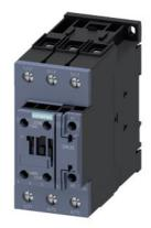
power contactor, AC-3 50 A, 22 kW / 400 V 1 NO + 1 NC, AC / DC 20-33 V, with varistor, 3-pole, Size S2, screw terminal
