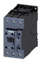
power contactor, AC-3 50 A, 22 kW / 400 V 1 NO + 1 NC, 110 V AC, 50 Hz, 3-pole, Size S2, screw terminal
