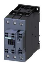
power contactor, AC-3 40 A, 18.5 kW / 400 V 1 NO + 1 NC, 24 V AC 50 Hz, 3-pole, Size S2, Spring-type terminal
