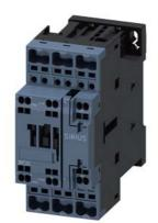
power contactor, AC-3 25 A, 11 kW / 400 V 1 NO + 1 NC, 24 V AC, 50 Hz 3-pole, Size S0 Spring-type terminal
