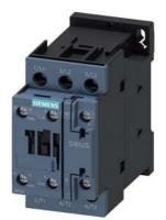
power contactor, AC-3 25 A, 11 kW / 400 V 1 NO + 1 NC, 110 V AC, 50 Hz, 3-pole, Size S0 screw terminal
