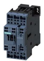
power contactor, AC-3 17 A, 7.5 kW / 400 V 1 NO + 1 NC, 24 V DC 3-pole, Size S0 Spring-type terminal
