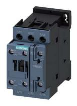
power contactor, AC-3 9 A, 4 kW / 400 V 1 NO + 1 NC, 110 V AC, 50 Hz 3-pole, Size S0 screw terminal
