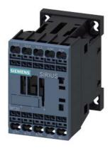
Power contactor, AC-3 16 A, 7.5 kW / 400 V 1 NC, 24 V DC 3-pole, Size S00 Spring-type terminals
