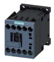
Power contactor, AC-3 16 A, 7.5 kW / 400 V 1 NC, 24 V DC 3-pole, Size S00 screw terminals
