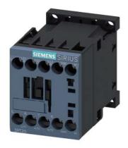
Power contactor, AC-3 16 A, 7.5 kW / 400 V 1 NC, 24 V AC, 50/60 Hz 3-pole, Size S00 screw terminals
