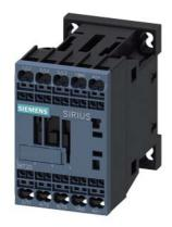
power contactor, AC-3 12 A, 5.5 kW / 400 V 1 NO, 24 V DC 3-pole, Size S00 Spring-type terminal
