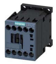
Power contactor, AC-3 12 A, 5.5 kW / 400 V 1 NC, 230 V AC, 50 / 60 Hz 3-pole, Size S00 screw terminal
