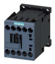
Power contactor, AC-3 12 A, 5.5 kW / 400 V 1 NC, 24 V AC, 50 / 60 Hz 3-pole, Size S00 screw terminal
