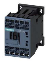
Power contactor, AC-3 9 A, 4 kW / 400 V 1 NC, 230 V AC, 50 / 60 Hz 3-pole, Size S00 Spring-type terminal
