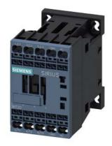
Power contactor, AC-3 9 A, 4 kW / 400 V 1 NO, 230 V AC, 50 / 60 Hz, 3-pole, Size S00 Spring-type terminal
