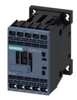
Power contactor, AC-3 9 A, 4 kW / 400 V 1 NC, 110 V AC, 50 / 60 Hz 3-pole, Size S00 Spring-type terminal
