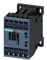
Power contactor, AC-3 9 A, 4 kW / 400 V 1 NO, 110 V AC, 50/60 Hz 3-pole, Size S00 Spring-type terminal
