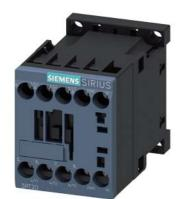
Power contactor, AC-3 9 A, 4 kW / 400 V 1 NC, 230 V AC, 50 / 60 Hz 3-pole, Size S00 screw terminal
