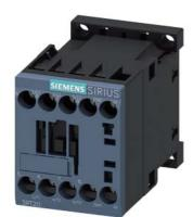
Power contactor, AC-3 9 A, 4 kW / 400 V 1 NC, 110 V AC, 50 / 60 Hz 3-pole, Size S00 screw terminal
